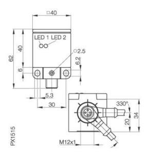
**Inductive Sensors** BES Q40KFU-PSC15A-S04G-M01 40 x 40 x 62 normally-open Sn=15mm shielded Factor 1, magnetic field immune, diagnostic
